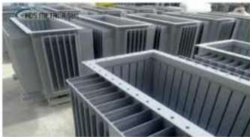
Fig:- Transformer Tank
